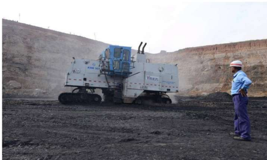
Dust Suppression - Surface Miner at Koyagudem OC of SCCL
