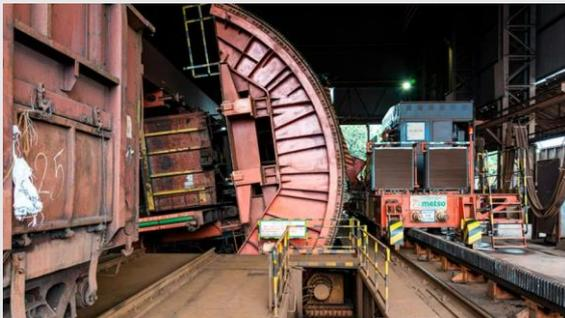
The wagon tippler assisted in tipping incoming material from wagons into the apron feeder for easier stacking. Simultaneously, the shifter mechanism was built and installed so that the racks could be switched to an outward line parallel to the inward line after emptying.
