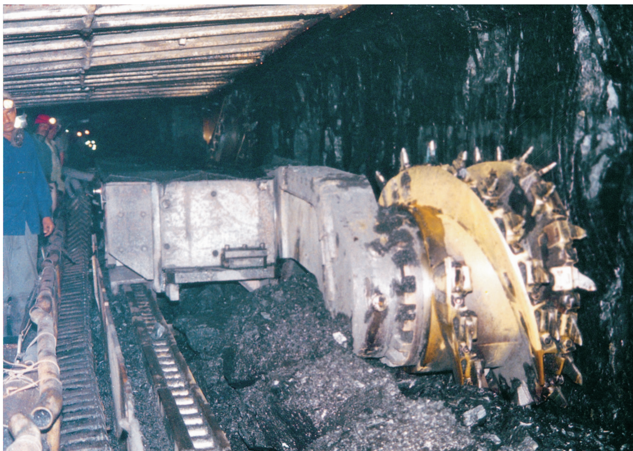
Shearer with Longwall support – a coal mining machine in an under ground mine
