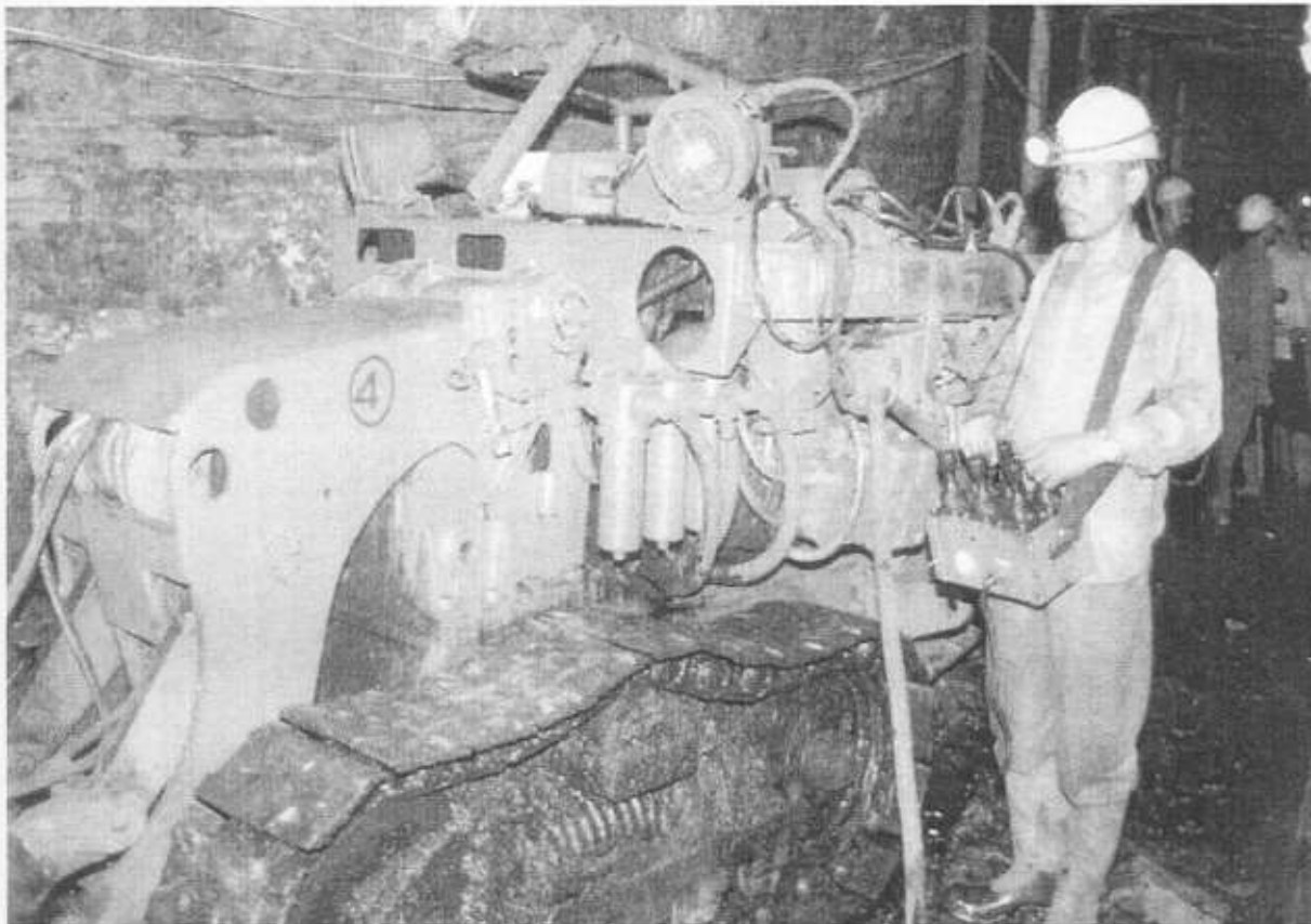
Hydraulic Side Discharge Loader is being operated in an underground mine
